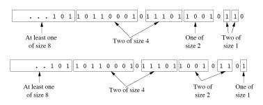
Bit stream divided into buckets following DGIM rules (top), with new 1 arriving (bottom)
