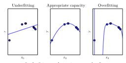
Left: Linear functions underfit Center: Polynomials of degree 2 neither under- nor overfit Right: Polynomials of degree 9 overfit
